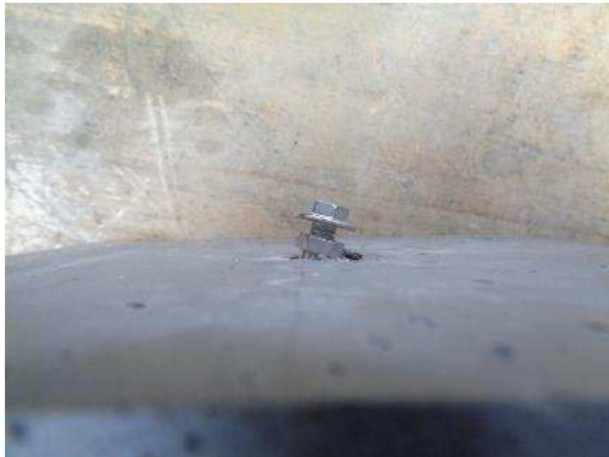
Photo No. 15 Typical Shear Anchor Withdrawal Failure Mode Detail
