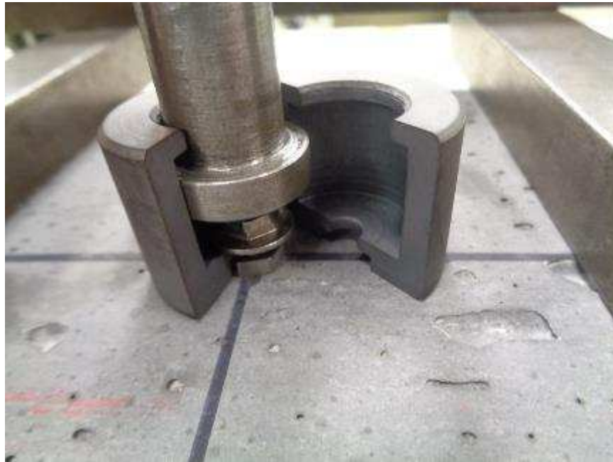
Photo No. 7 Typical Tensile Fixture Setup Detail
