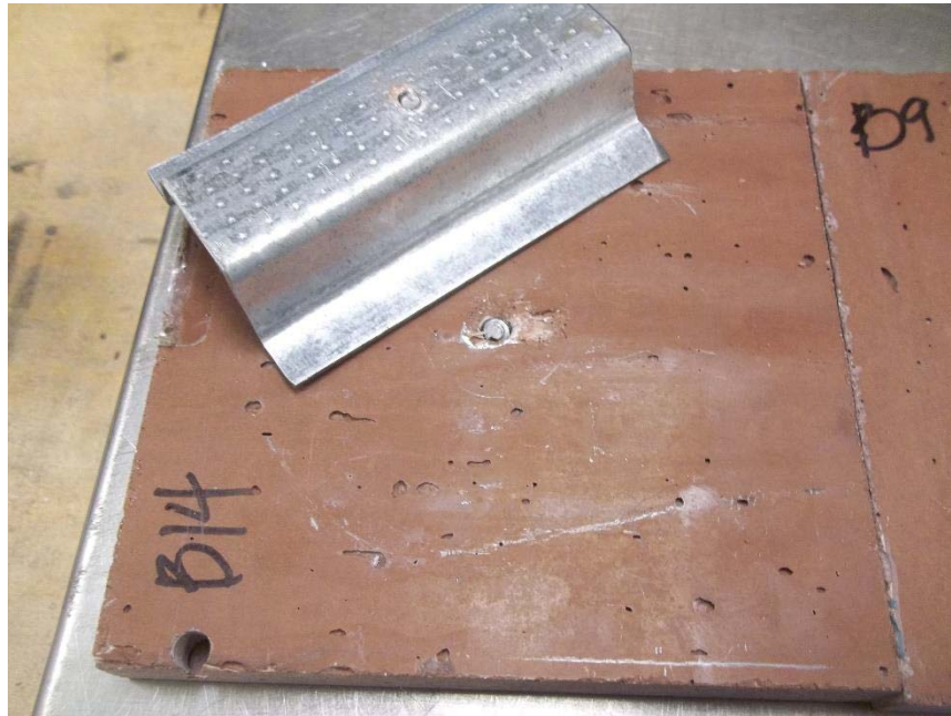
Photo No. 7 Representative Shear Specimen Fastener Shear Failure Mode Detail
