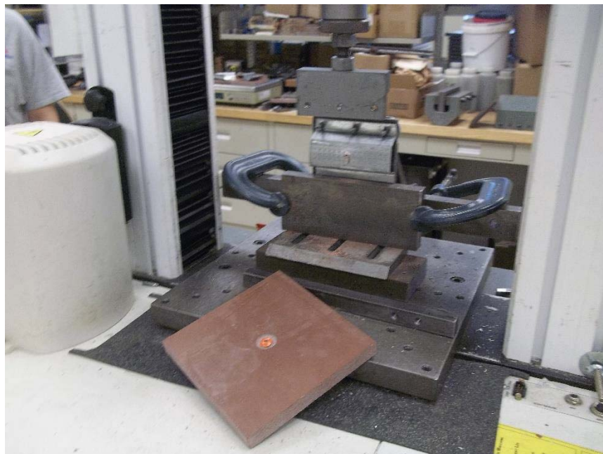
Photo No. 6 AISI S905 Fastener Evaluation – Depiction of Representative Shear Load Specimen Failure
