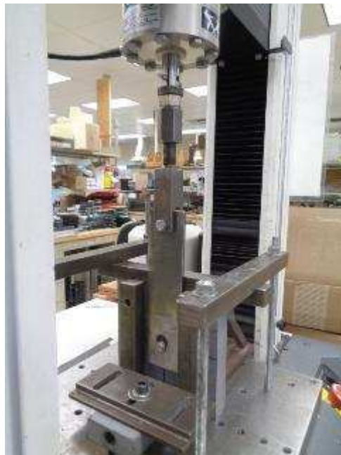
Photo No. 12 Typical Shear Test Setup Detail
