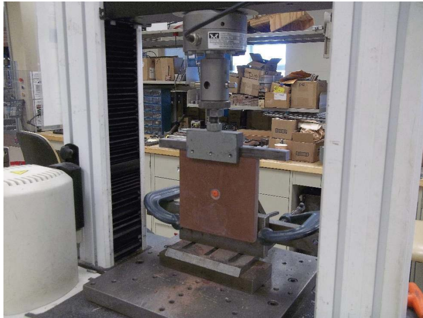
Photo No. 5 AISI S905 Fastener Evaluation - Shear Load Evaluation Setup
