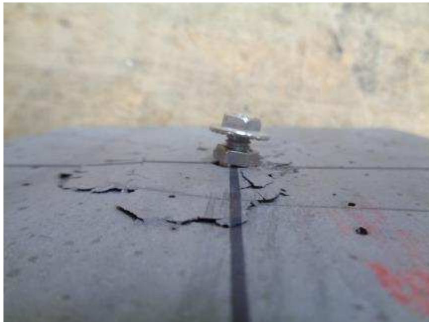
Photo No. 14 Typical Shear Concrete Pullout Failure Mode Detail
