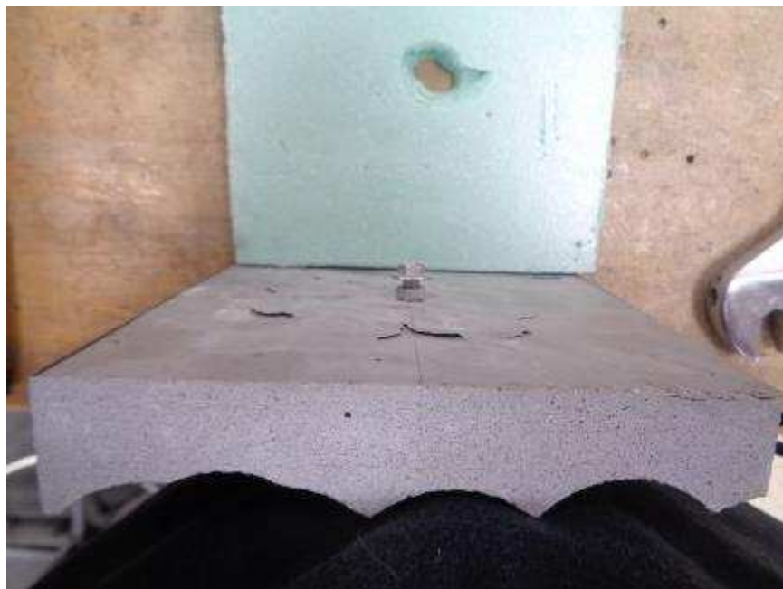
Photo No. 10 Typical Block B Tensile Concrete Pullout Failure Mode Detail
