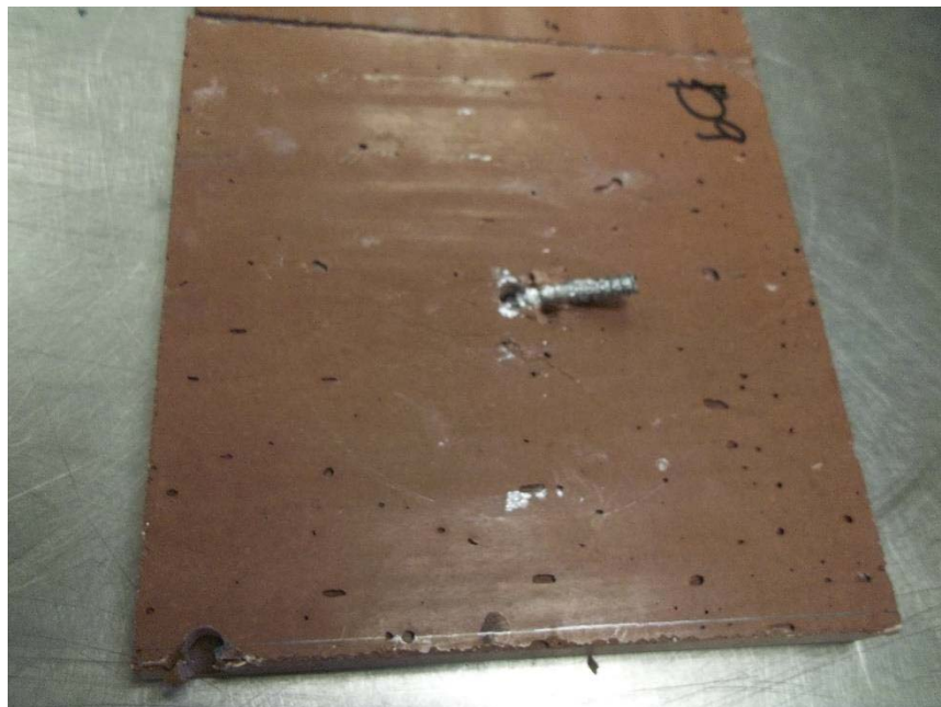
Photo No. 8 Shear Specimen Fastener Tile and Pull-Out Failure Mode Detail
